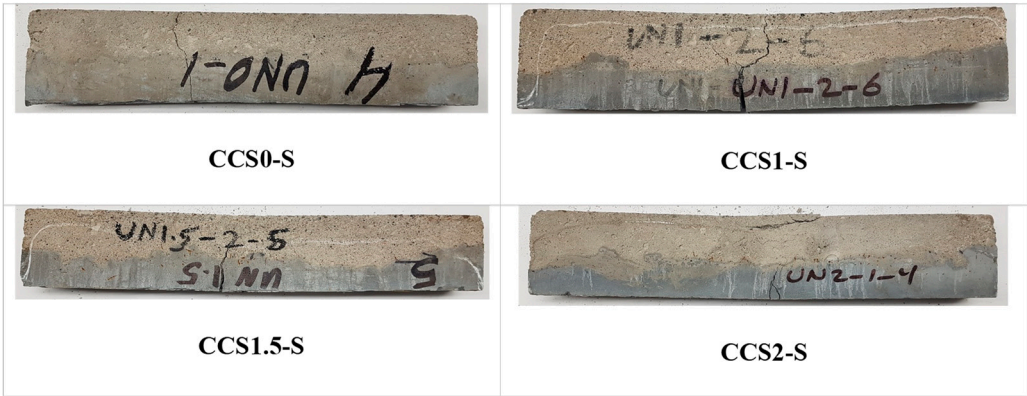
Figure 4. Cracking patterns for CCS flexural prisms.
