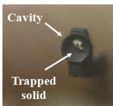
Figure 7. Unlike microwave treatment, direct calcination of LED fails to sufficiently recover the chip from the reflective cavity. The photo was taken using a magnifying loupe.
