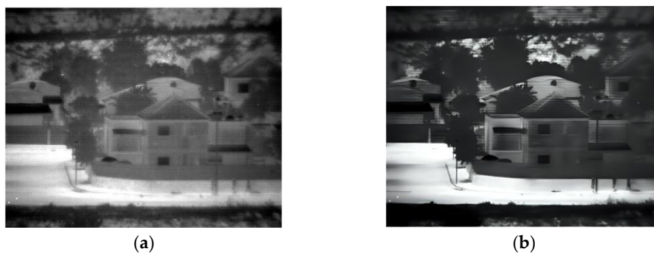
Figure 9. Low-light images in 150 Kelvin. (a) original image; (b) after enhancement
