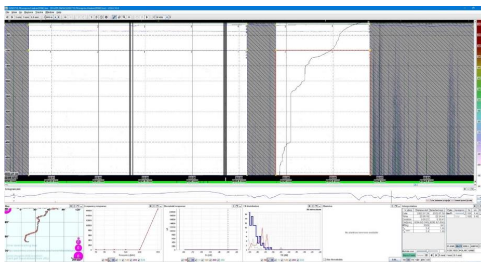
Figure 2. Scrutinizing of the 38 kHz Simrad EK80 recordings using the LSSS post processing software. Screen dump from the LSSS after post processing of a five nautical mile distance along the 41° W longitude from the North Pole to the transect. Shaded areas removed because of noise, and 641 of 3320 pings used for final allocation of S_A – values to the different species groups (here plankton in the upper 100 m layer and mesopelagic/plankton in the deeper layer).
