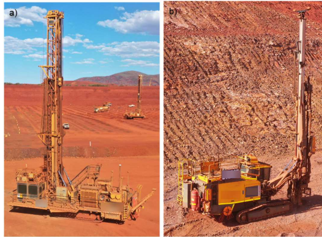
Figure 1. Examples of blasthole drill rigs used for collecting MWD data [49]: a) Terex SKS 12, utilized for the drilling of 0.229m production blast holes and b) Epiroc D65, used in the creation of 0.165m wall control blast holes.
