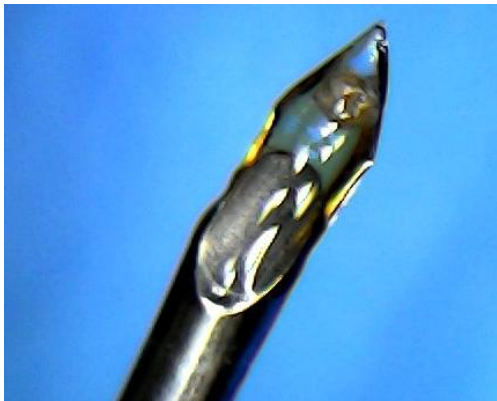
Figure 6. Fragment of the uranium mineral from APB-11 at the tip of the sample holder for analysis at beamline I18 at the Diamond Light Source.
