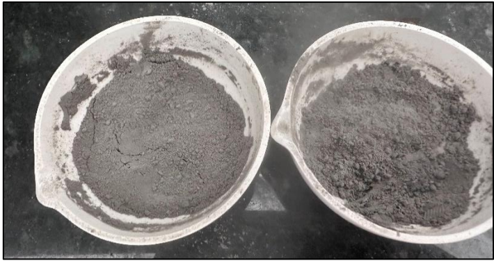
Figure 8. Final sample. After the processes of cutting, grinding, calcination at 500°C, crushing, and a second calcination at 600°C.
