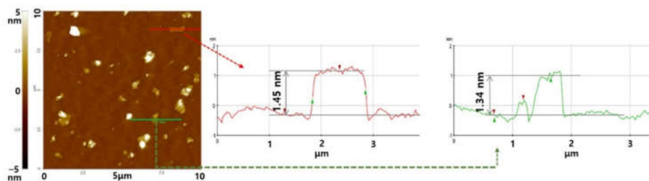
Figure 2. AFM non-contact mode image and line profiles of CMG + on a Si wafer substrate.
