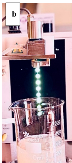
Figure 1. Alginate Microbead Production Process (a) Schematic Representation of Alginate-Enzyme Bead Formation Process; (b) Buchi Encapsulator Setup for Microbead Formation.
