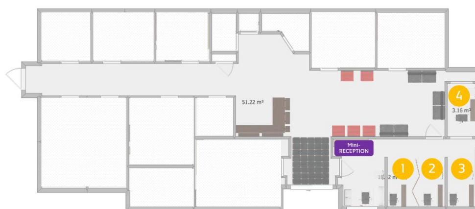
Figure 4. Schematic diagram of the remodelled COVID-19 vaccination area. Instead of having patients travel between seven consulting rooms in the clinic, patients can receive their COVID-19 vaccinations in a dedicated area. By repurposing the conference room and children's play area, we allowed for a mini reception area that led to four vaccination stations.
