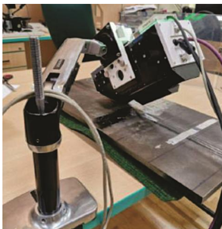
Figure 7. Measuring device PULSTEC U-X360 for the XRD method.
