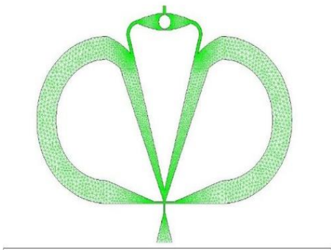
Figure 4. The mesh used for the simulations of geometry in Fluent.
