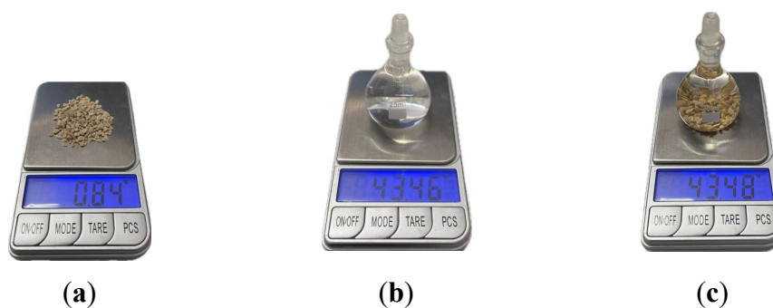
Figure 3. Kernel density determination by pycnometer method: (a) weight of seeds ( m_1 ); (b) weight of water and pycnometer ( m_2 ); (c) weight of seeds, water, and pycnometer ( m_3 ).
