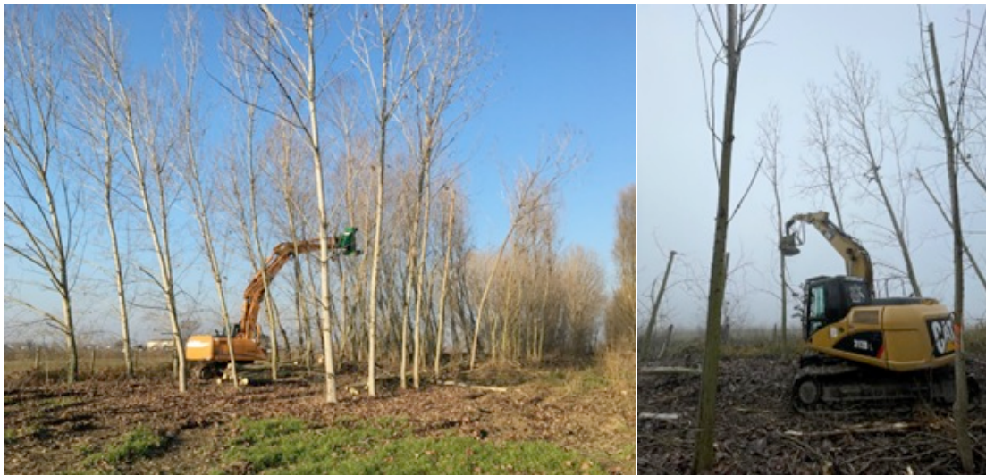
Figure 2. The two machines at work: to the left, the shears; to the right, the disc-saw.
