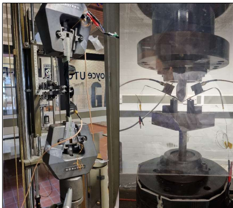
Figure 2. Sensor positions for the tensile test (left) and 3-point bend (right).
