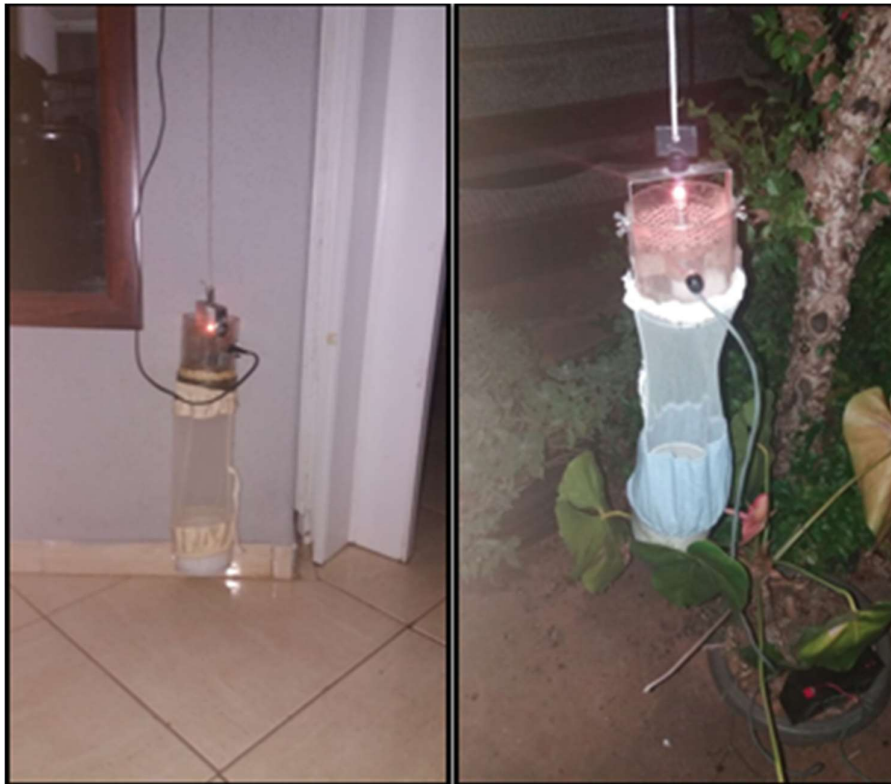
Figure 1. CDC type light traps, installed inside (left) and outside (right) the residences in the study.
