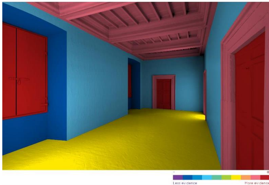
Figure 5. View of the reconstructive model with a scale depicting historical evidence. Colors applied to each RU correspond with different amount of evidence.
