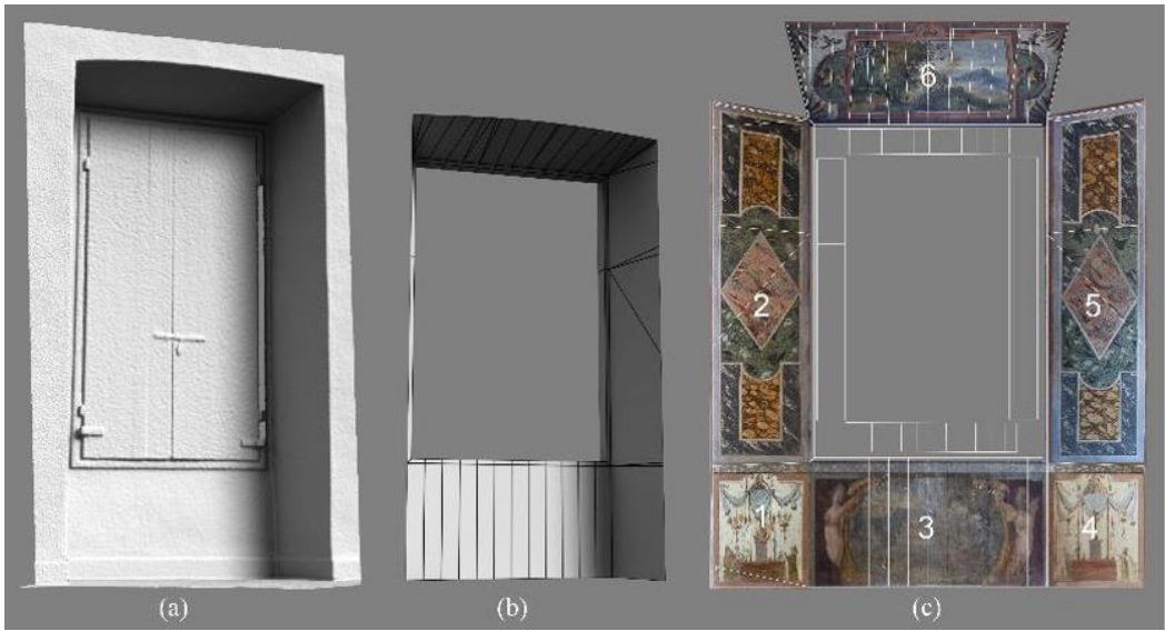
Figure 13. (a) 3D model of the system consisting of the intrados and its corresponding window (from the Galleria ), (b) reconstructive model of the intrados ( Quarto Camerino ), (c) texture of the reconstructive model.
