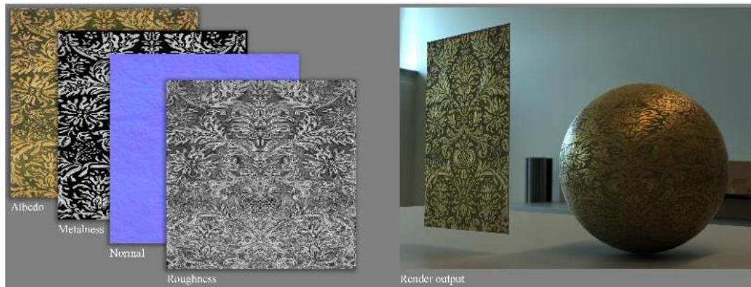
Figure 16. Set of textures aimed at simulation the optical behavior of leather sheets (metallic and dielectric) and their simulation using ambient lighting generated by an HDR image.
