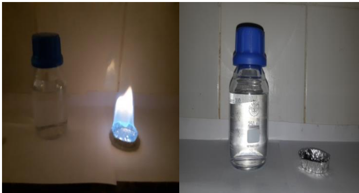
Figure 5. Characteristics of ethanol produced from TCW: flame (left), colorless liquid (right).
