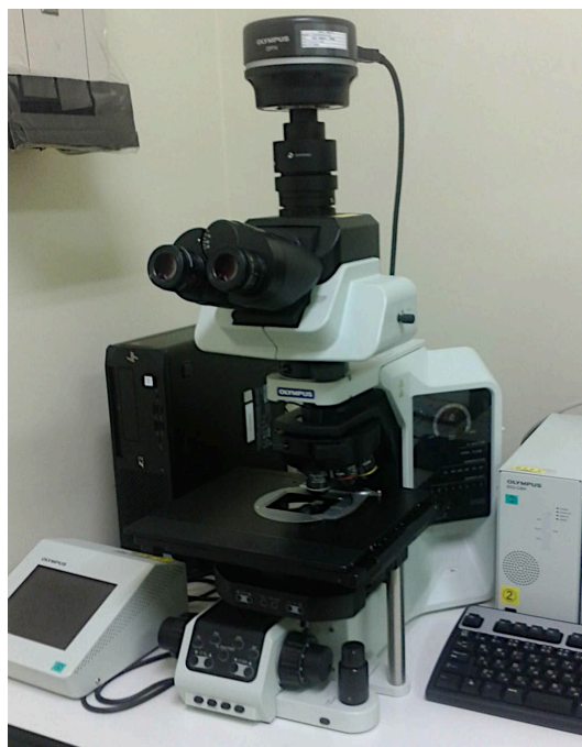
Figure 17. Olympus upright microscope. The hematoxylin and eosin (H&E) and immunohistochemical slides were evaluated using a conventional upright microscope (Olympus BX63).
