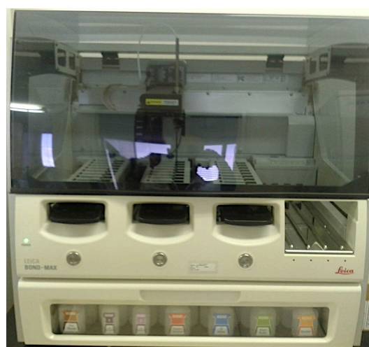
Figure 11. Automated immunohistochemistry staining system. The immunohistochemical staining were performed using a fully automated immunohistochemistry and in situ hybridization staining system following the manufacturer's instructions (Leica BOND-MAX).
