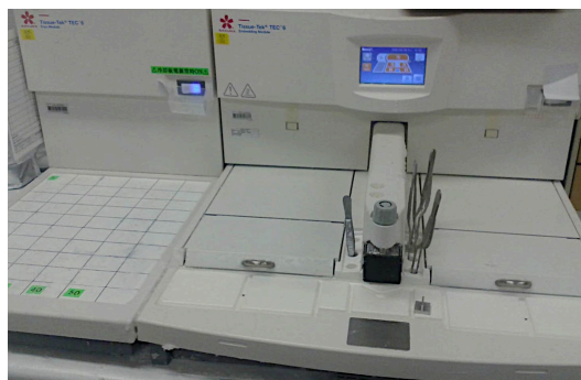
Figure 7. Tissue embedder. The processed tissue was embedded in paraffin, forming paraffin blocs for sectioning using a tissue embedder (Tissue-Tek® TEC™ 6 Embedding Console System).
