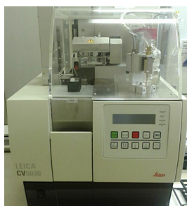
Figure 12. Glass coverslipper for immunohistochemical tissue slides. Coverslipping was achieved using a Leica CV5030 fully automated glass coverslipper.
