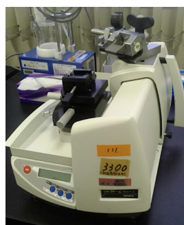
Figure 8. Automated slide stainer. Paraffin blocks were trimmed at 2\mu\text{m} using a Yamato REM-710 microtome.
