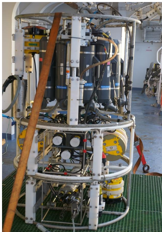
Figure 1. Carousel water sampler used for the measurements at sea. The SBE 9 + CTD profiler is located at the bottom with the first pair of CT sensors. The second pair (not visible on this photo) is located at the top. The pump and the pipe connecting it to the conductivity sensor are visible in the foreground.
