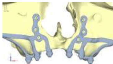
Figure 9. (a) Design of the subperiosteal implant on the upper jaw model V3; (b) Upper jaw model V3 with optimized front section with additional screws, stress on frontal screws remained unchanged.
