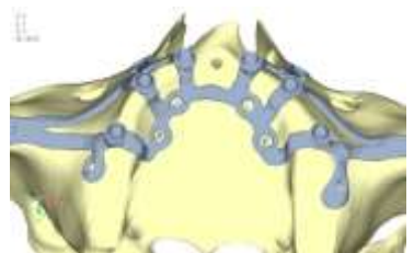
Figure 6. Design of the upper jaw model V2 structure using screws placed posteriorly in the vestibular direction rather than the palatal direction.
