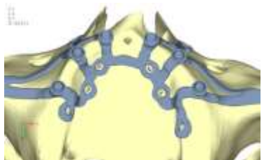
Figure 4. Design of the subperiosteal implant on the upper jaw model V1 with added posterior screws, reducing stress on anterior parts and achieving more balanced distribution.
