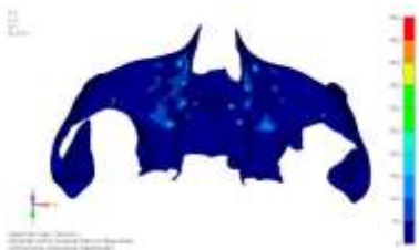
Figure 3. Model V0 with the least critical load configuration 2 distributed across the posterior teeth.
