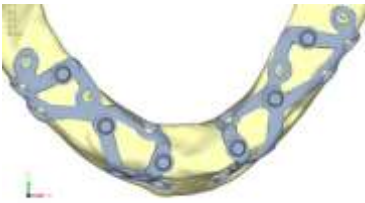
Figure 24. (a) Design of the subperiosteal implant on the lower jaw model V3; (b) Decreased stress loading on the material of the model V3.
