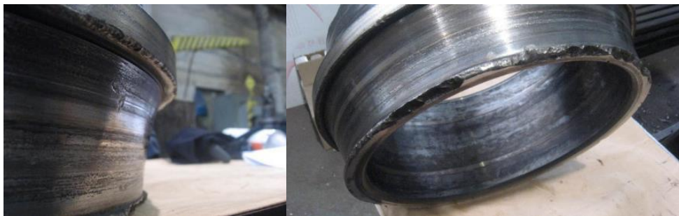
Figure 8. Signs of peeling and damage to the raceway and side surfaces of the inner ring.
