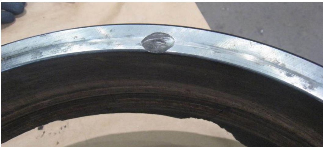
Figure 9. Signs of damage to the side surfaces of the outer ring.
