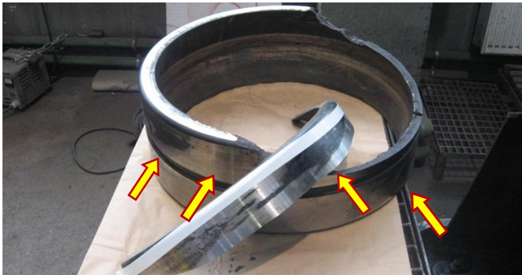
Figure 11. Fretting corrosion on the bearing's outer ring mating surface.
