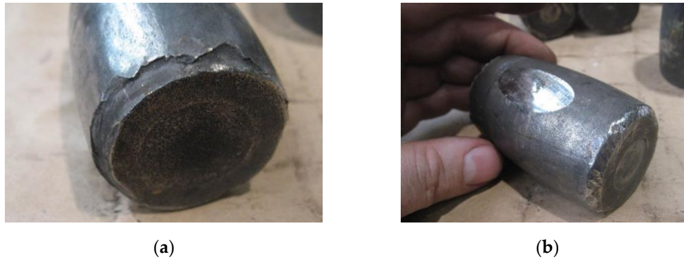
Figure 10. Damage to the bearing's rolling elements: (a) chipped contact surface between the rolling element and the raceway, (b) chipped edge of the rolling element.
