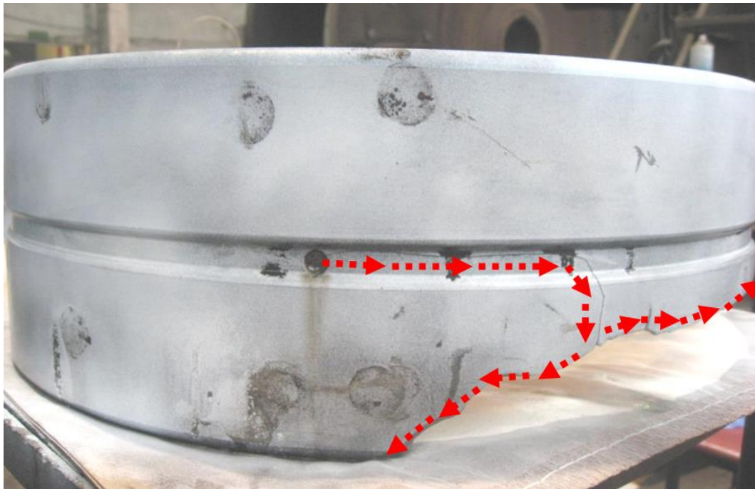
Figure 15. Direction of crack propagation.
