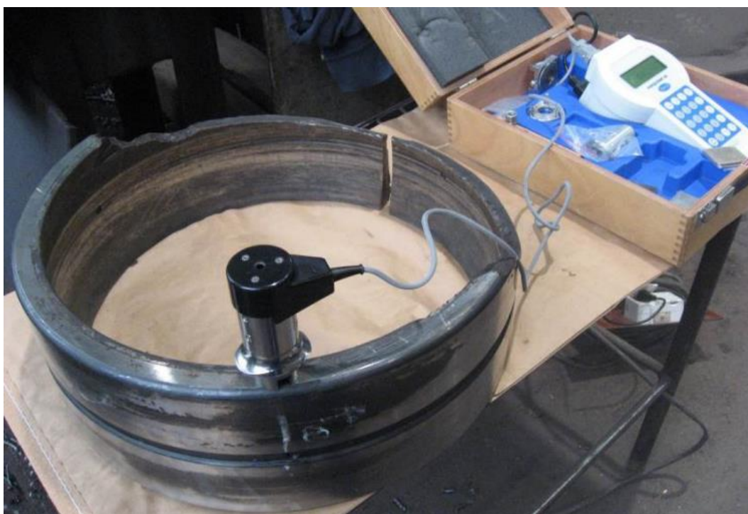
Figure 4. The measurement of hardness of the damaged outer ring of the bearing using the COMPUTEST S.C. hardness meter.
