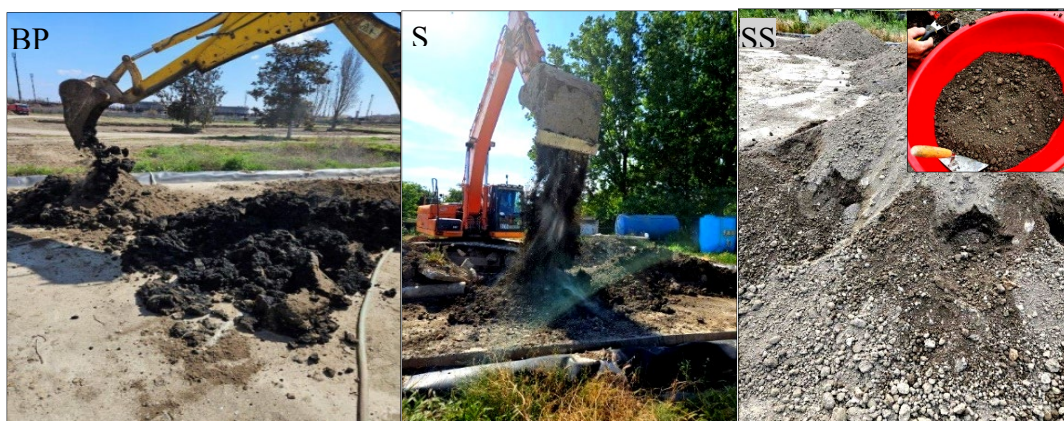
Figure 1. Bioremediation experiment of petroleum-contaminated soil treated with sludge Biopile (BP); soil aeration (SA); soil sampling (SS).
