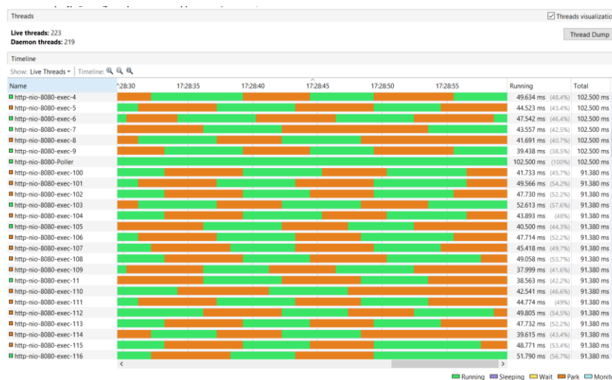
Figure 19. Resources usage for the fully synchronous approach.
