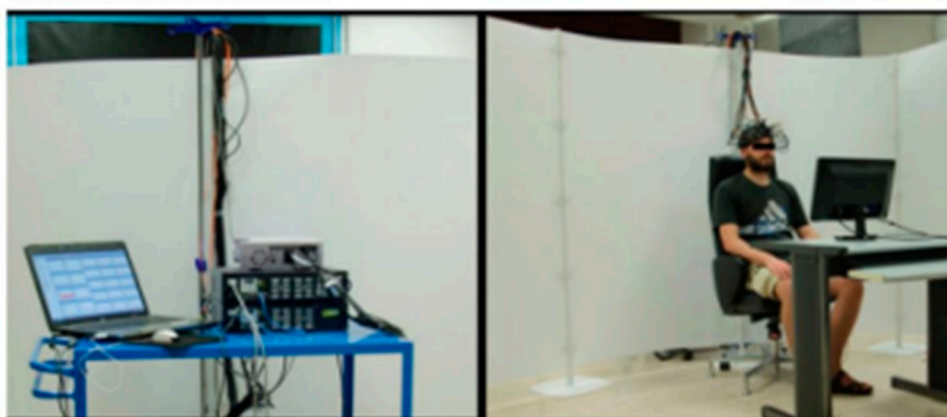
Figure 3. Functional near infrared spectroscopy (fNIRS) in an experimental setting. The subject is seated comfortably in a chair with a high back. In order to fit the size and shape of the head, the lighting and collecting optical fiber bundles are combined into a flexible probe holder that is fastened to the head using a Velcro brand fastener (Quaresima & Ferrari, 2019).
