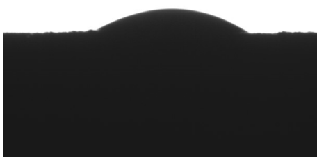
Figure 4. Contact angle measurement. Contact angle measurement showing hydrophilicity of the CA-treated wood.
