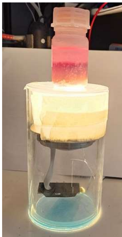
Figure 1. Self designed photolysis unit for photochemical experiments. The units consist of two Plexiglas tubes into which a commercially available LED ceiling spotlight (light temperature 7400 K).
