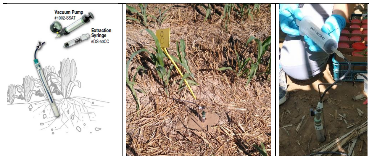
Figure S3. Ceramic suction cups. Installation in the field and extraction of the soil solution.
