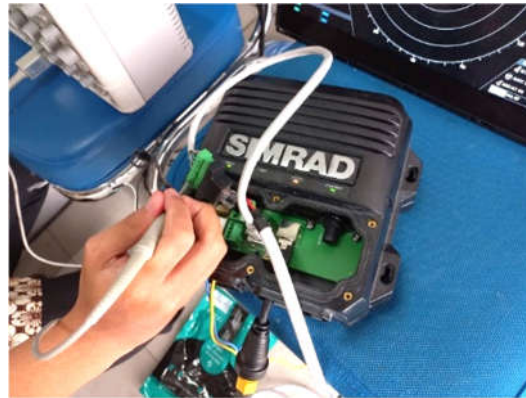
Figure 4. Measurement and Data Collection of Pins on The Compressed Pulse Radar Pulse Radar [Personal Documents].
