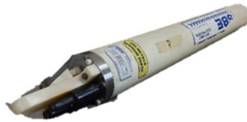
Figure 3. SBE26 Plus to measure sea level using seawater pressure & temperature sensor.
