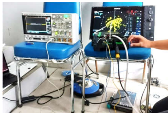
Figure 5. Retrieval of signal data from each pin on The Compressed Pulse Radar complex using Spectrum Analyzer and SIMRAD [Personal Documents].
