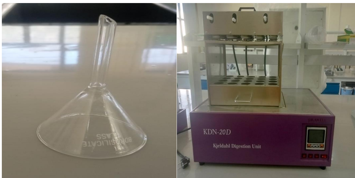
Figure 7. Funnel and Kjeldahl digester unit.
