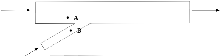
Figure 7. The key points for on-ramp merging area
