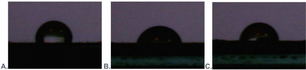
Figure 11. The representing images of the droplets of water exhibiting the contact angles for assessed layer coatings. A) support; B) alginate; C) alginate–perfluorooctyl.
