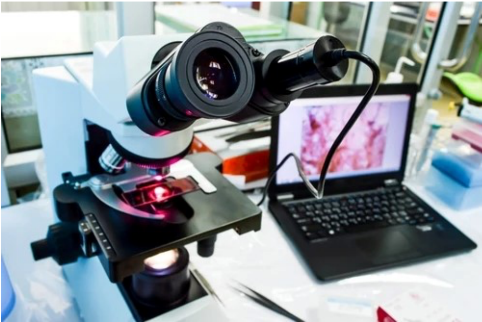
Figure 2. Microscope integrated with a CCD camera system for real-time data collection and analysis.
