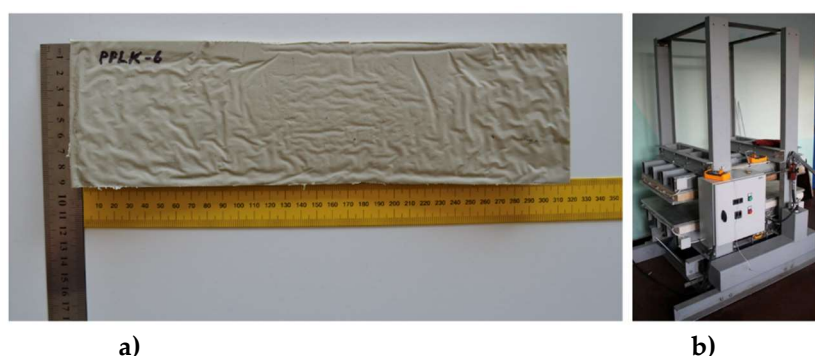
Figure 5. The laboratory specimen PPLK-6 a) and the hot press b) were used for the specimen preparation.
