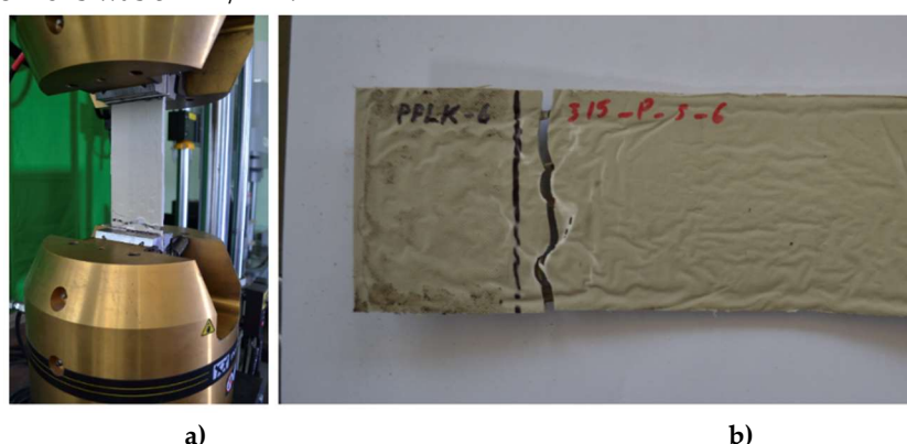
Figure 6. Testing the laboratory composite specimen: a) - testing device INSTRON 8802; b) - laboratory composite specimen PPLK-6 after it collapses.
