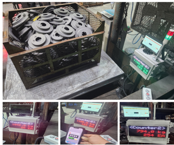
Figure 11. This is an image of the test result showing the product counting accuracy.
