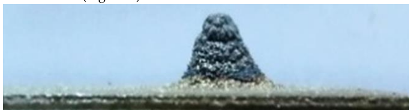
Figure 3. Metallization figure produced by stationary microplasma spraying of zirconium wire onto a stationary steel substrate for 10 seconds [29].
