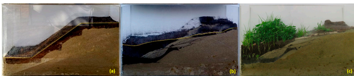
Figure 19. The variation in the profile of a sandy excavation protected by 5 cm of OS (with seeds) during rainfall simulation at different periods: (a) t = 0 minutes, (b) t = 10 minutes, and (c) after approx.—four months, during the winter.
