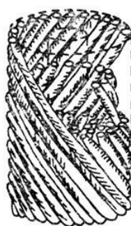
Figure 2. Spiral arrangement of macrofibrils in layers [31].
