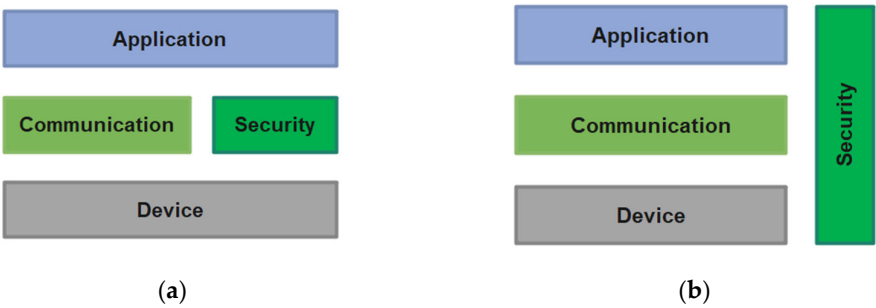
Figure 1. (a) The three-layer architecture of IoT [11]; (b) The three-layer architecture with its security.
