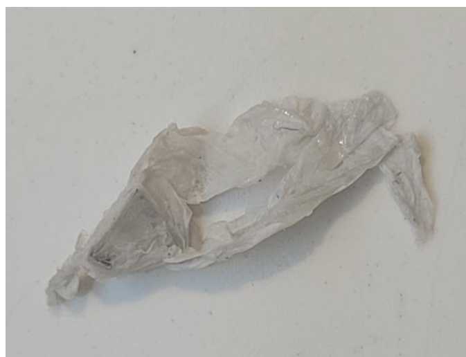
Figure 2. Photograph of the polymer (C_2H_4O-C_2H_4)_x appearance after extraction of tantalum powder and DMSO elimination from the Sample 1.
