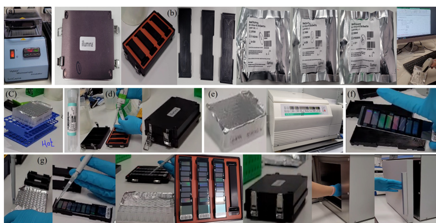
Figure A21. Representation of the lab work for BeadChip DNA Hybridisation: (a) Incubate the MSA1 plate in the oven at 95°C for 20 minutes to denature the DNA. (b) Assemble the hybridisation chambers. (c) Allow the plate to cool down. (d) Add 200 \mu l of buffer (PB2) to the top and bottom of the BeadChip reservoirs, then cover it. (e) Centrifuge the MSA1 plate. (f) Place the three BeadChips into their inserts. (g) Transfer 26 \mu l from the MSA1 plate to each section of the BeadChip, close the lid, and incubate at 48°C overnight.
