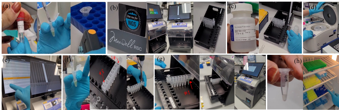
Figure A16. Representation of the lab work for DNA extraction using the Maxwell instrument. (a) Add 10 \mu l of RNase A solution to the sample and incubate for 5 minutes. (b) Manual preparation of the Maxwell FFPE cartridge: Open the Maxwell instrument. Place the cartridges to be used in the deck tray. For each cartridge, place a plunger into well # 8. For each cartridge in the deck tray, place an empty elution tube. (c) Add 50 \mu l of Nuclease-Free Water to the elution tube. (d) Centrifuge the incubated DNA for 5 minutes. (e) Select the type of tissue used for Maxwell to extract DNA (FFPE in this case). (f) Transfer the blue part of the sample containing DNA into well # 1. (g) It takes 40 minutes for the Maxwell to extract the DNA. (h) Take the samples and store them in the fridge. The water and the DNA are visible in the tube.
