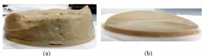
Figure 6. Filter cakes formed by the base WBDF (a), GO/NC-WBDF (b).
