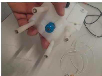
Figure 1. Cylindrical Sensor with 3mm Diameter inside the Blue Gland (XMS-310 with 10 MHz bandwidth).
