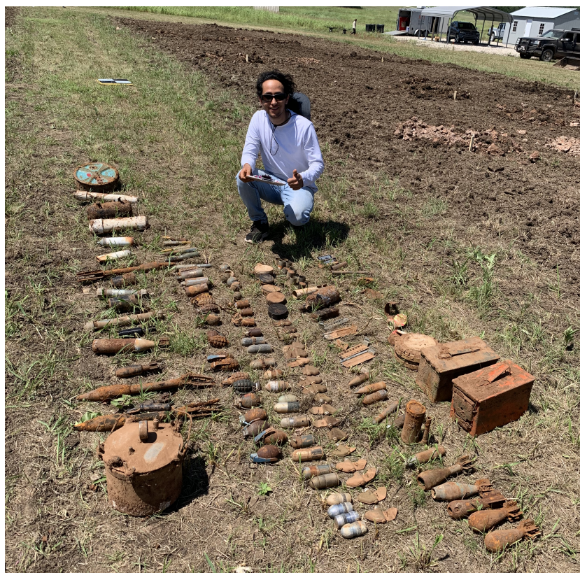
Figure 5. Excavated objects from the test field being verified after the data was collected from all the metal detectors.
