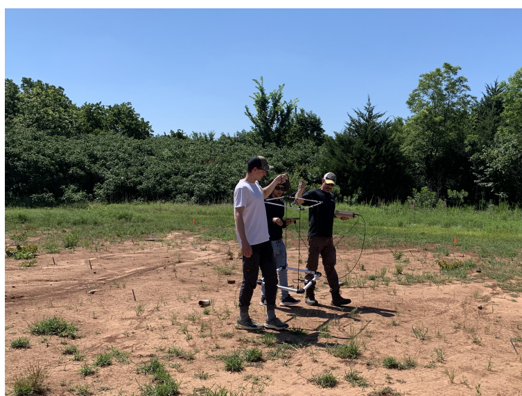
Figure 4. Test field demonstrating the data collection procedure from the EM61 Lite: being carried by two people with another person simultaneously analyzing peak responses and marking those locations in the test field.
