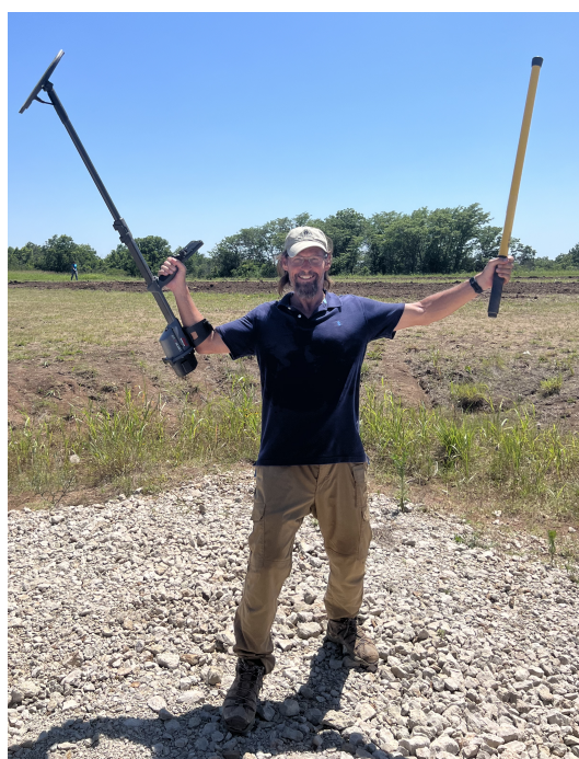
Figure 3. Handheld metal detectors used to detect landmines and UXOs in our test field. In the photo, CTX 3030 held in right hand and ML-3S held in left hand.
