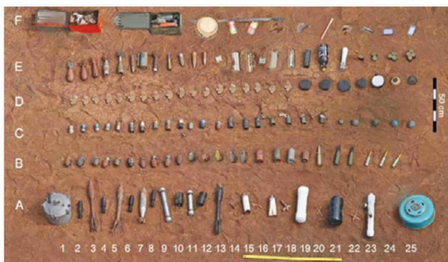
Figure 1. Condensed picture of test field showing different landmines and their arrangement in lines A to F from north to south, with A1 facing east and A25 in the west [21].
