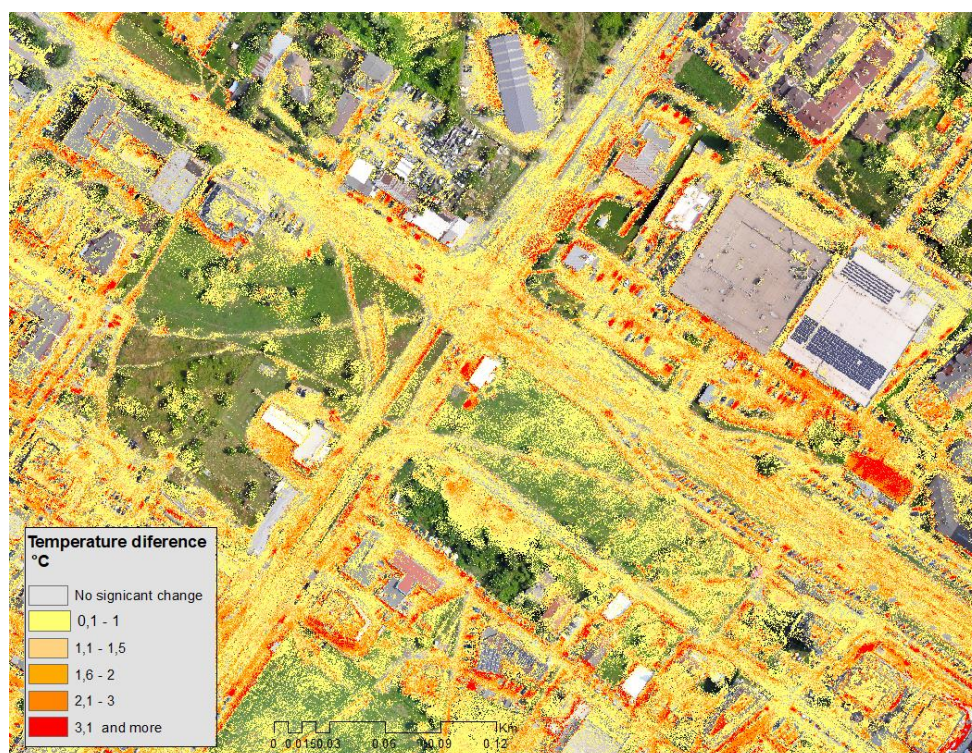
Figure 17. Temperature differences on land surfaces (°C) between 11.07-17-07.2024, Sofia City, Lyulin residential complex.
