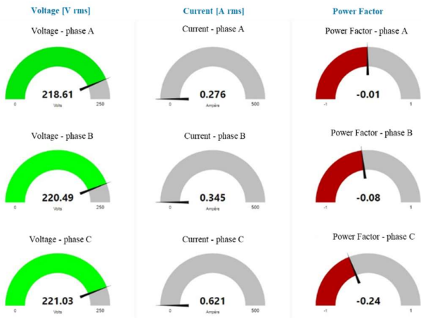
Figure 10. Measurements (voltage, current, and power factor) at the low voltage buses of the distribution system – obtained via IEC 61850.
