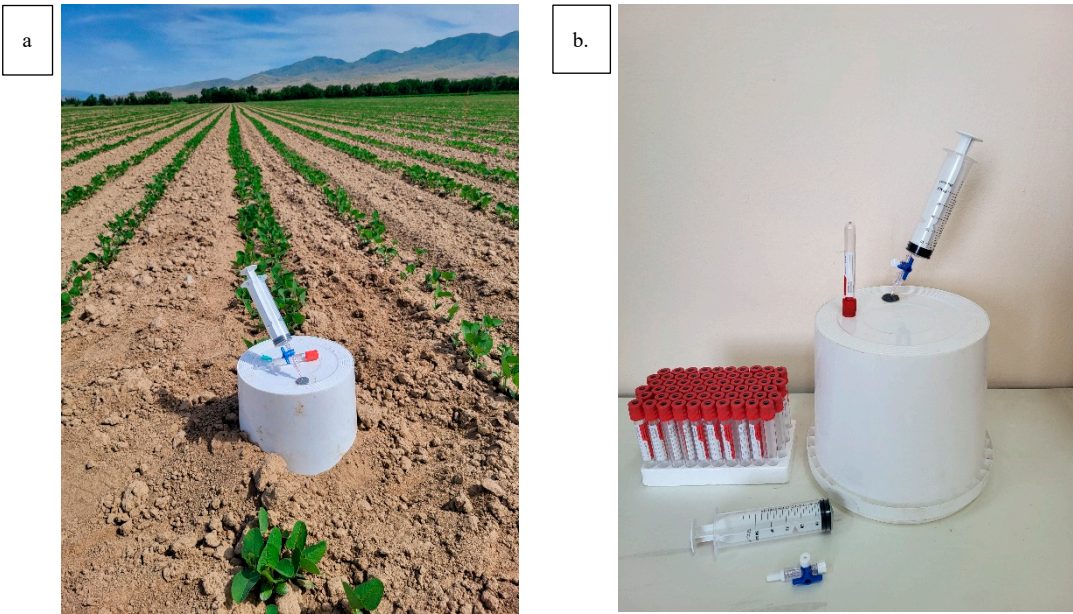
Figure 2. Gas Sampling Using the Closed Chamber Method: (a) Overview of the Chamber; (b) Installation of the Chamber at the Field Site.
