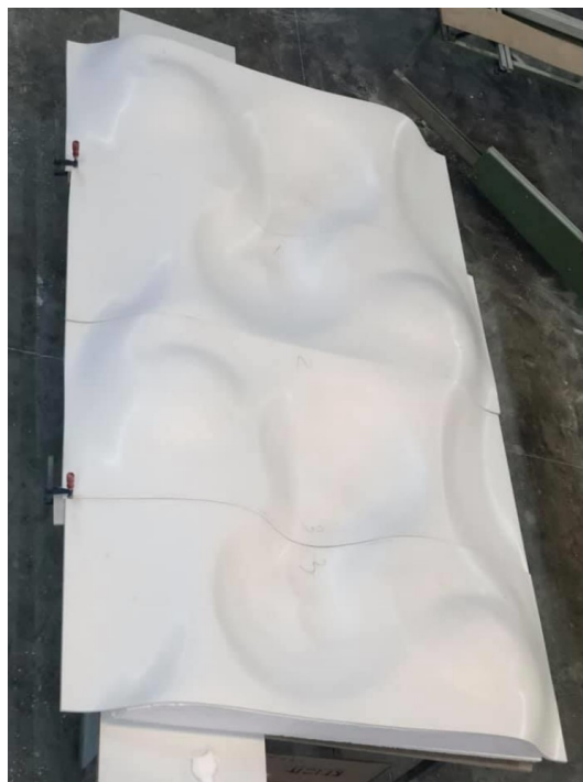
Figure 7. Combination final termoforming piece. Same piece rotate 180° generating different shapes.
