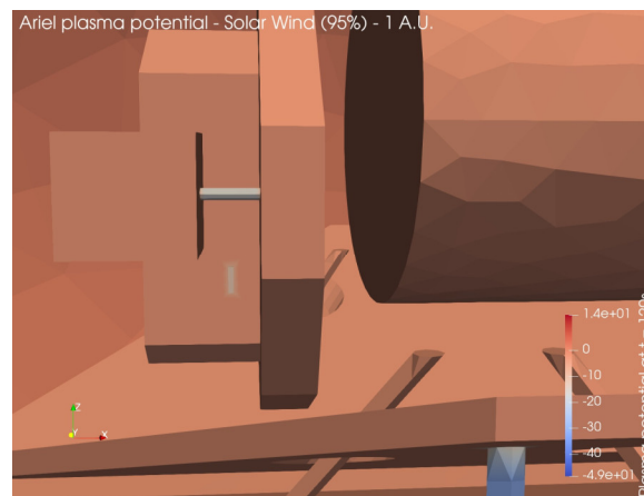
Figure 20. 3D map of plasma potential – Solar Wind (1 A.U.) – 95% conditions: closeup on FPE-IC connector and FPE strut.
