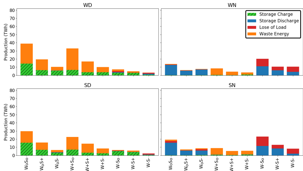
Figure 7. Behavior of storage using the sequential model in the INT_ALT case. Periods with discharge losses are shown in red, while wasted energy is indicated in yellow.
